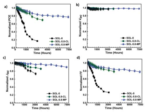
Fig. 5 Evolution of J-V parameters (a) PCE, (b)  $V_{\rm oc}$ , (c)  $J_{\rm sc}$ , and (d) FF for the different devices measured at different periods over ten months. Devices are always stored and measured under ambient laboratory conditions (T = 22-25 °C, and RH = 25–55% RH).
