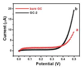
Fig. 8 /-V curves of (a) the bare GC and (b) GC-2 in the presence of 250  $\mu$ M urea in 0.1 M PBS (pH = 7.0).
