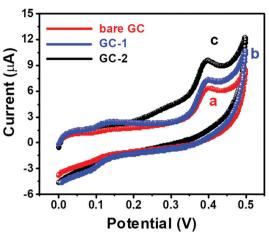
Fig. 7 CV curves of (a) the bare GC, (b) GC-1 and (c) GC-2 in the presence of 250  $\mu$ M urea in 0.1 M PBS (pH = 7.0) at an applied scan rate of 0.1 V s<sup>-1</sup>.
