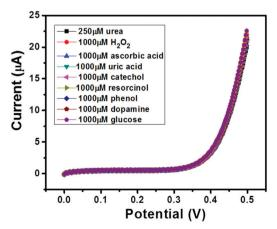
Fig. 11 I-V curves of **GC-2** in the presence of urea (250  $\mu$ M) in 0.1 M PBS (pH = 7.0) with different interfering species (1000  $\mu$ M).
