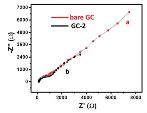
Fig. 6 Nyquist plot of (a) the bare GC and (b) **GC-2** in 2 mM  $[Fe(CN)_6]^{3-/4}$  solution in 0.1 M PBS (pH = 7.0).
