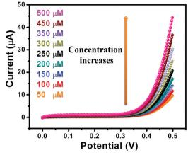
Fig. 9 I-V curves of GC-2 in different concentrations (50-500  $\mu$ M) of urea in 0.1 M PBS (pH = 7.0).
