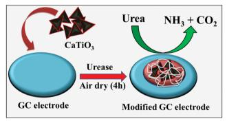
Scheme 2 Schematic illustration of urea sensing
