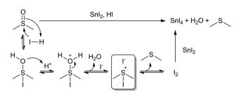
Scheme 1  $I_2$ -Mediated mechanism of Sn(II) oxidation in DMSO. A possible intermediate species, iododimethylsulfonium iodide, is highlighted inside the square.
