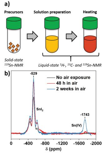
Fig. 1 (a) Steps of tin-based perovskite material preparation studied in this work as possible sources of Sn(II) oxidation; (b) solid-state 119Sn-NMR spectra of Snl<sub>2</sub> precursor with and without air exposure.
