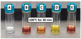
Fig. 3 (a) <sup>1</sup>H-NMR spectra of FASnI<sub>3</sub> and MASnI<sub>3</sub> in DMSO at 1 M after heating the solutions at 100 °C for 30 min. The green arrow highlights the peak of DMS originating from heating the solution; (b) vials containing different solutions before and after being heated at 100 °C for 30 min. A: FAI in DMSO; B: SnI2 in DMSO; C: FASnI3 in DMF; D: FASnI3 in DMSO with 10 mol% SnF2; E: CsSnI3 in DMSO.
