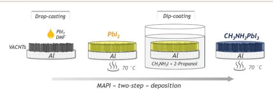
Fig. 1 Scheme of the two-step process used for MAPI deposition
