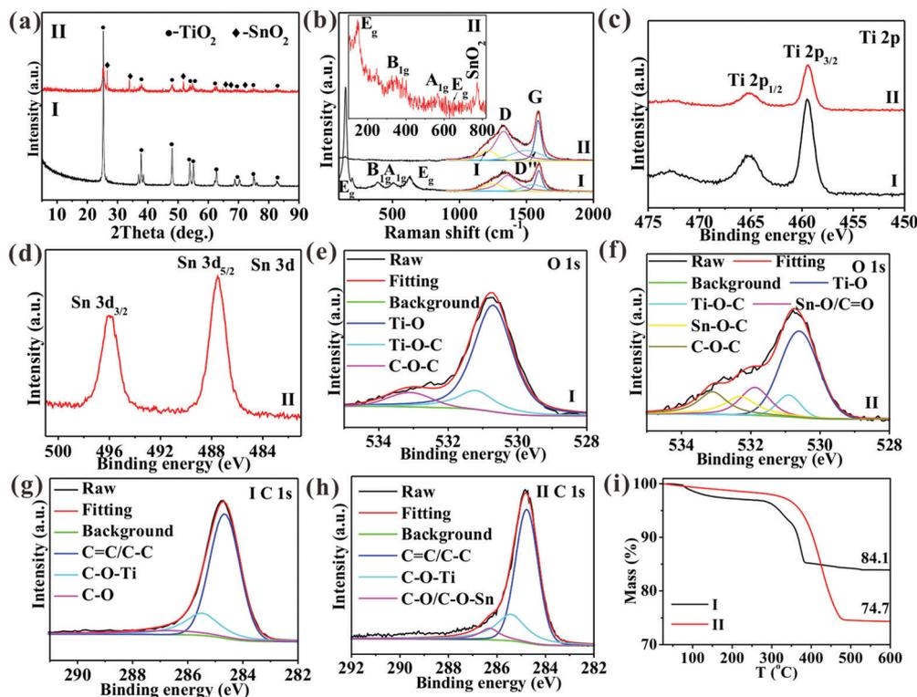
Fig. 2 (a) XRD, (b) Raman spectra, (c–h) XPS spectra of Ti 2p (c), Sn 3d (d), O 1s (e and f), and C 1s (g and h), and (i) TG curves of TiO<sub>2</sub>/C (I) and SnO<sub>2</sub>@TiO<sub>2</sub>/C (II).
