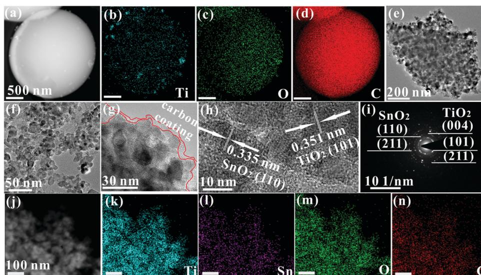
Fig. 3 (a) High angle annular dark field image and the corresponding EDS elemental mapping images of Ti (b), O (c), and C (d) of TiO<sub>2</sub>/C spheres; (e) TEM image of crushed TiO<sub>2</sub>/C spheres; (f) TEM image, (g and h) HRTEM image, and (i) the corresponding SAED pattern of SnO<sub>2</sub>@TiO<sub>2</sub>/C; and (j) HAADF image and the corresponding EDS elemental mapping images of Ti (k), Sn (l), O (m), and C (n) of SnO<sub>2</sub>@TiO<sub>2</sub>/C.
