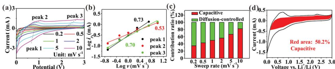
Fig. 6 (a) CV curves at different scanning rates; (b) the line relationship of  $\log(i)$  vs.  $\log(\nu)$  at peaks 1–3 marked in (a); (c) the percentages of the pseudocapacitive contribution at different scanning rates; and (d) the detailed pseudocapacitive contribution at a scanning rate of 1 mV s<sup>-1</sup> of SnO<sub>2</sub>@TiO<sub>2</sub>/C.
