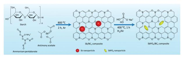
Fig. 1 Schematic illustration of the preparation process for the  $SbPO_4/BC_x$  composite.
