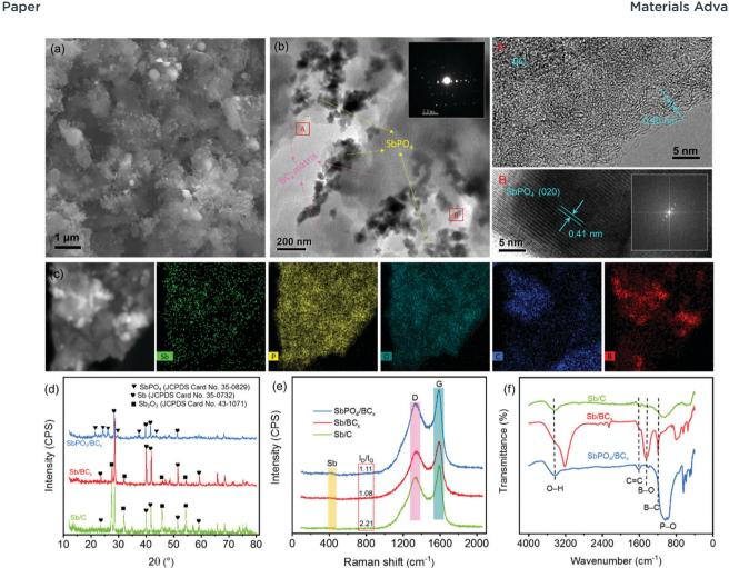
Fig. 3 SEM image (a), TEM and HRTEM images (b), and scanning TEM image with the corresponding EDS mappings of the Sb, P, O, C and B elements (c) of the SbPO<sub>4</sub>/BC<sub>x</sub> composite; (d) XRD patterns, (e) Raman spectra and (f) FT-IR spectra of the SbPO<sub>4</sub>/BC<sub>x</sub>, Sb/BC<sub>x</sub> and Sb/C samples. The two insets present the SAED pattern and the FFT pattern of the HRTEM image.
