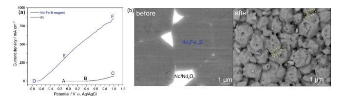
Fig. 1 (a) LSV of a Pt-wire working electrode (black curve) and a sintered Nd-Fe-B magnet (blue curve) with 0.6 mol  $L^{-1}$  FeSO<sub>4</sub>, 0.4 mol  $L^{-1}$ (NH<sub>4</sub>)<sub>2</sub>SO<sub>4</sub>, 0.175 mol L<sup>-1</sup> Na<sub>3</sub>Cit and 0.4 mol L<sup>-1</sup> H<sub>3</sub>BO<sub>3</sub> in the electrolyte, at a scan rate of 100 mV s<sup>-1</sup>. (b) BSE–SEM images of the magnet before and after LSV.
