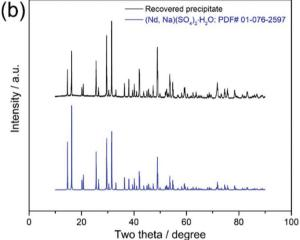
Fig. 3 (a) BSE-SEM images with an inset of a real image and (b) XRD pattern of the REE precipitates.
