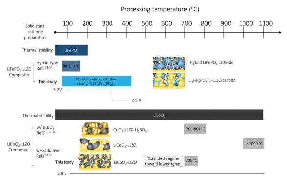
Fig. 6 Overview of the cathode composite design and ceramic processing choices of all-oxide Li-garnet SSBs based on LiFePO<sub>4</sub>- and LiCoO<sub>2</sub>-based cathode composites: processing temperature vs. chemical and mechanical stability
