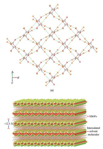
Fig. 1 Perspective view of 1EG as representative showing (a) the 2D halogen-organic frameworks constructed by the Br...O halogen bonding interactions (green dashed lines) and (b) the supramolecular structure.
