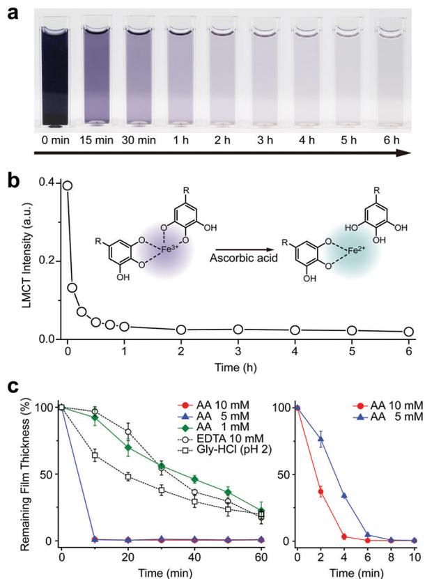
**Fig. 1** (a) Time-lapse optical images of the Fe<sup>3+</sup>-TA MPC solution after addition of ascorbic acid at 0 min (10 mM). (b) Graph of LMCT intensity at 565 nm versus reaction time. (c) Graphs of film thickness versus reaction time. The Fe<sup>3+</sup>-TA MPC film was incubated in an aqueous solution of AA (1, 5, or 10 mM), EDTA (10 mM), or gly-HCl buffer (pH 2). The right graph for AA (5 and 10 mM) is the enlarged one for the first 10 min of incubation.
