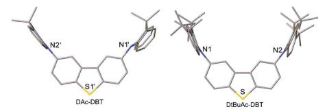
Fig. 2 X-ray crystal structures of DAc-DBT and DtBuAc-DBT.
