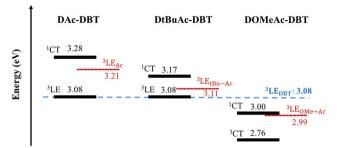
Fig. 6 A schematic energy diagram of DAc-DBT, DtBuAc-DBT and DOMeAc-DBT. All energies are given in eV and were calculated from the onsets of the corresponding spectra in zeonex films, compared with their individual D and A moieties. No indication of <sup>3</sup>CT states is obtained in DAc-DBT and DtBuAc-DBT from calculations, neither are they observed in our experiments, therefore, their <sup>3</sup>CT states are not represented in this
