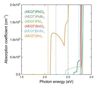
Fig. 4 Calculated optical absorption spectra for layered hybrid perovskites: (AEQT)PbCl<sub>4</sub>, (AEQT)PbBr<sub>4</sub>, (AEQT)Pbl<sub>4</sub>, (AEQT)SnCl<sub>4</sub>, (AEQT)SnBr<sub>4</sub> and (AEQT)SnI<sub>4</sub>, where the vertical dash lines are the corresponding fundamental direct band gaps.
