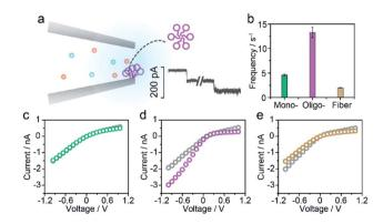
Fig. 3  $\,$  A $\beta$ 1–42 oligomer sensing with glass nanopores. (a) The typical step like current fluctuations induced by the adsorption of A $\beta$ 1–42 oligomers onto the nanopore sidewall. (b) Frequencies of the pulse-like signals for the sensing of three types of A $\beta$ 1–42 peptides. I-V curves of the glass nanopore measured in the pure electrolyte before (gray) and after A $\beta$ 1–42 monomer (c), oligomer (d) and fibre (e) sensing, respectively.
