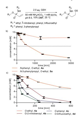
Fig. 2 (a) Reaction of glutathione (GSH) with differently substituted vinylphosphonamidates. 10 mM vinylphosphonamidates were reacted with 20 mM GSH at pH 8.5 (NH<sub>4</sub>HCO<sub>3</sub> buffer). Concentration of the starting materials over time, mean and error from three independent measurements, monitored by UPLC-UV. (b) N-Phenyl vs. N-alkyl comparison. (c) Comparison of different O-substituents. Dotted line depicts 50% conversion.
