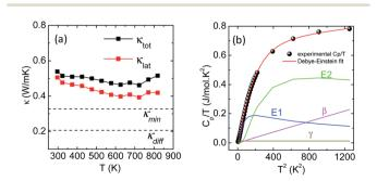
Fig. 2 (a) Total (black) and lattice (red) thermal conductivity of pristine AgPbBiSe<sub>3</sub>. (b)  $C_{\rm p}/T$  vs.  $T^2$  plot within the 2–30 K range. The red line is the fit produced using the combined Debye–Einstein model. The individual contributions from electronic ( $\gamma$ ), Debye ( $\beta$ ) and the two Einstein terms ( $E_1$  and  $E_2$ ) are also plotted.
