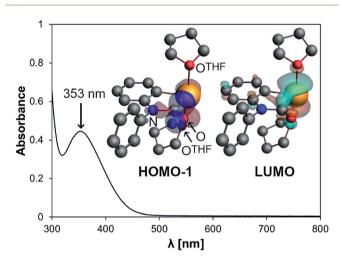
Fig. 3 UV/vis spectrum of 2 (0.4 mM solution in THF) and orbitals involved in the transition at 353 nm according to TD-DFT calculations on  $[Bi(CONPh(C_6H_4))(thf)_2]^+$ .
