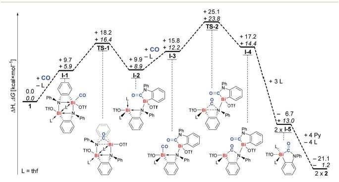
Scheme 3 Proposed mechanism for reaction of 1 with CO to give insertion product 2;  $\Delta H$  values (regular font) and  $\Delta G$  values (italic) are given in kcal  $mol^{-1}$ . L = thf.
