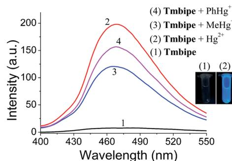
**Fig. 1** Fluorescence spectra of **Tmbipe** in the absence and presence of Hg<sup>2+</sup>, MeHg<sup>+</sup> or PhHg<sup>+</sup>. [**Tmbipe**] = 10 μM; [Hg<sup>2+</sup>] = [MeHg<sup>+</sup>] = [PhHg<sup>+</sup>] = 20 μM. The inset shows the aqueous solution photograph of **Tmbipe** in the absence and presence of Hg<sup>2+</sup> under UV light irradiation.
