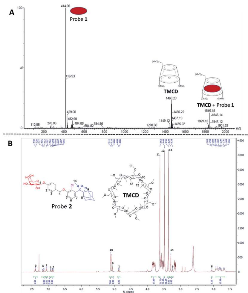
Fig. 4 (A) Negative ESI spectra of an aqueous solution of probe **1** and TMCD prepared in a 1 : 1 molar ratio. (B)  $^1\text{H-NMR}$  spectrum of the crystalline supramolecular complex of probe **2** with TMCD. The crystallization experiment was carried out in  $\text{H}_2\text{O} : \text{DMF}$  (95 : 5) with probe **2** and TMCD mixed at an initial molar ratio of 1 : 5.
