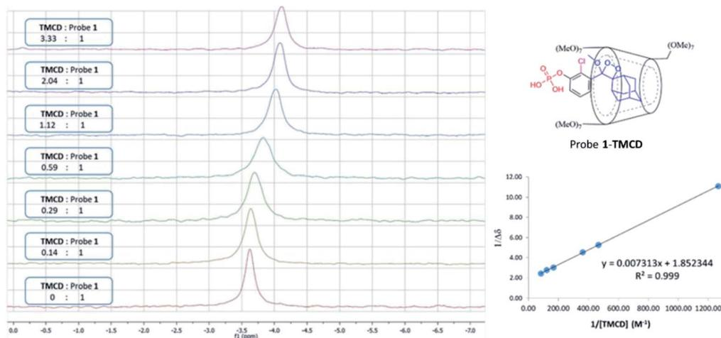
Fig. 5 (Left)  $^{31}\text{P}$ -NMR titration experiment of TMCD and probe 1. Conditions: 500  $\mu\text{L}$  of  $\text{D}_2\text{O}$ , 5 mg of probe 1 and up to 50 mg of TMCD. (Right) Correlation of  $1/\Delta\delta$  as a function of probe  $1/[\text{TMCD}]$ , based on the Benesi-Hildebrand equation.
