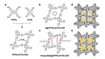
Scheme 1 (a) Schematic of the synthesis of TFPPy-ETTA-COF. (b) Physical isolation of sulfur (S<sub>8</sub> ring) in the COF. (c) Covalent engineering of polysulfide chains on the pore walls. (d) Graphic of S<sub>8</sub> (yellow) loaded in S@TFPPy-ETTA-COF. (e) Graphic of polysulfide chains locked in polysulfide@TFPPy-ETTA-COF (one-layer polysulfide is shown for clarity; yellow; polysulfide).
