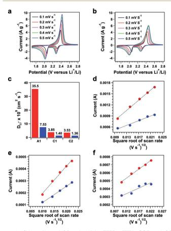
Fig. 6 CV profiles of (a) polysulfide@TFPPy-ETTA-COF and (b) S@TFPPy-ETTA-COF at different scanning rates. (c) Li<sup>+</sup> ion diffusion coefficients of polysulfide@TFPPy-ETTA-COF (red) and S@TFPPy-ETTA-COF (blue). The plots of current *versus* square root of the scanning rate of the (d) anodic peak (A1), (e) cathodic peak C1, and (f) cathodic peak C2 for polysulfide@TFPPy-ETTA-COF (red) and S@TFPPy-ETTA-COF (blue).
