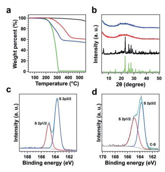
Fig. 3 (a) TGA curves of TFPPy-ETTA-COF (black curve), polysulfide@TFPPy-ETTA-COF (red), S@TFPPy-ETTA-COF (blue), and sulfur (green). (b) PXRD patterns of S@TFPPy-ETTA-COF (blue), polysulfide@TFPPy-ETTA-COF (red), a simple mixture of TFPPy-ETTA-COF and sulfur (black), and elemental sulfur (green). The XPS S2p spectra of (c) S@TFPPy-ETTA-COF and (d) polysulfide@TFPPy-ETTA-COF. A clear C-S band was identified.
