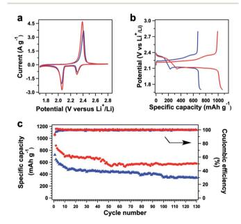
Fig. 5 (a) CV profiles of S@TFPPy-ETTA-COF (blue) and polysulfide@TFPPy-ETTA-COF (red) at a scan rate of 0.1 mV s<sup>-1</sup>. (b) Charge-discharge profiles of polysulfide@TFPPy-ETTA-COF (red) and S@TFPPy-ETTA-COF (blue) at 0.1C. (c) Cycling performances and coulombic efficiency of polysulfide@TFPPy-ETTA-COF (red) and S@TFPPy-ETTA-COF (blue) over 100 cycles at 0.1C.
