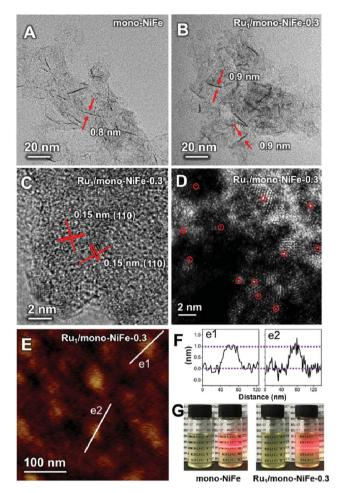
Fig. 1 TEM images of (A) mono-NiFe and (B)  $Ru_1/mono-NiFe-0.3$ ; (C) HRTEM image of  $Ru_1/mono-NiFe-0.3$ ; (D) HAADF-STEM image of  $Ru_1/mono-NiFe-0.3$  (the circles are drawn around some of the isolated Ru atoms); (E) AFM image of  $Ru_1/mono-NiFe-0.3$  nanosheets; (F) the corresponding height curves of AFM in (E); (G) photographs of the dispersion of mono-NiFe and  $Ru_1/mono-NiFe-0.3$  in water.
