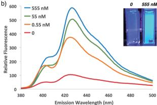
Fig. 7 (a) Schematic for the streptavidin detection assay. (b) Emission spectra and photographs of anthracene ATRP co-polymerization initiated from 7 following incubation with various concentrations of streptavidin by the protocol shown in (a). The spectra and photographs for various conditions were taken after 24 h of reaction time following excitation at 371 nm or by a hand-held UV lamp (365 nm).
