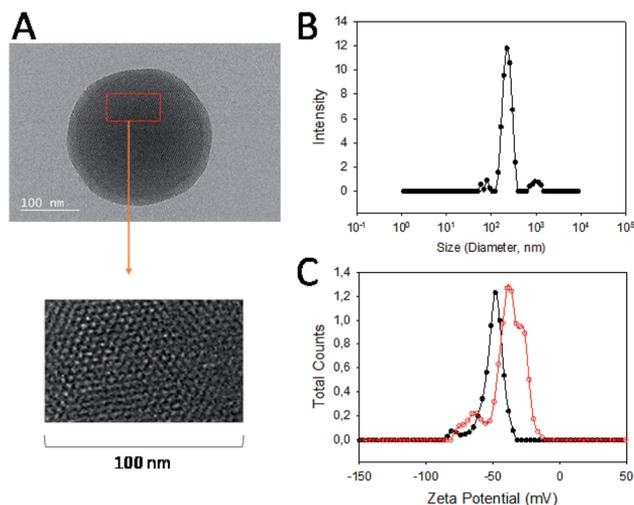
Fig. 1 Characterization of silica nanoparticles used in this study. (A) TEM analysis image of a typical particle after synthesis. The inset shows the ordered hexagonal pore structure on the surface of the particles. (B) DLS analysis of particle size after aptamer gate functionalization. (C) Stability analysis of epoxy and epoxy-aptamer grafted silica nanoparticles by zeta analysis.
