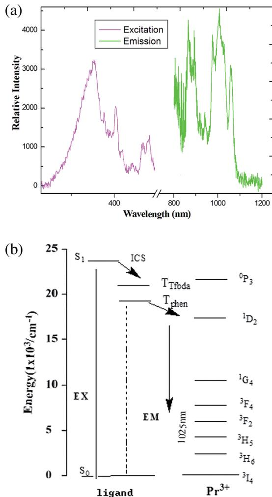
Fig. 5 (a) The excitation (monitored at  $\lambda_{em} = 980$  nm) and emission spectra ( $\lambda_{ex} = 376$  nm) of coordination polymer **1** in solid state. (b) Energy level scheme showing energy transfer processes in **1**.
