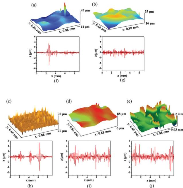
**Fig. 8** 3D profilometer images and line scanning curves of the MPU films. Surface area roughness of (a) MPU1, (b) MPU2, and (c) MPU3, (d) MPU4, and (e) MPU5 with  $R_q$  values of (a) 0.25, (b) 0.56, (c) 0.97, (d) 1.3, and (e) 2.3  $\mu\text{m}$ , respectively. Line roughnesses of (f) MPU1, (g) MPU2, (h) MPU3, (i) MPU4, and (j) MPU5, where the  $\lambda_a$  values are (f) 7.0, (g) 7.4, (h) 7.8, (i) 10.2, and (j) 12.9  $\mu\text{m}$ , respectively.
