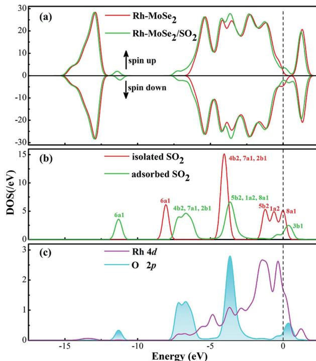
Fig. 10 DOS distribution of the Rh-MoSe<sub>2</sub>/SO<sub>2</sub> system. The dashed line is the Fermi level.
