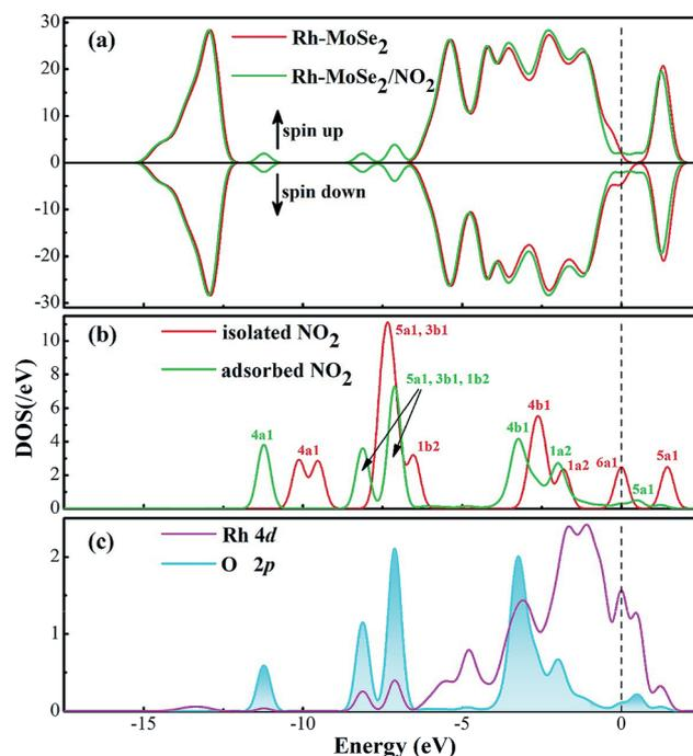
Fig. 8 DOS distribution of the Rh-MoSe<sub>2</sub>/NO<sub>2</sub> system. The dashed line is the Fermi level. In the gas DOS, the red value shows the orbitals of isolated molecules while the green one shows the orbitals of adsorbed molecules.
