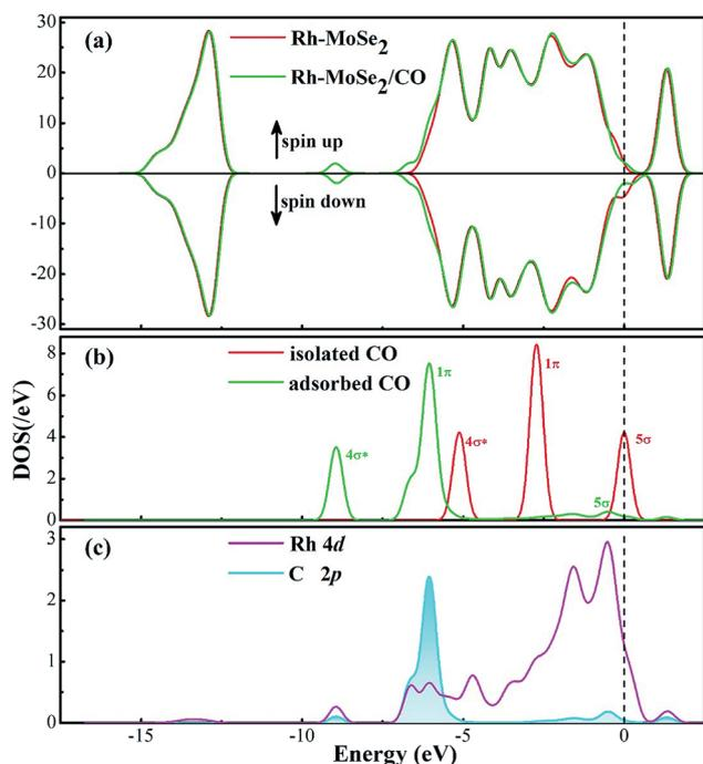
Fig. 4 DOS distribution of the Rh-MoSe<sub>2</sub>/CO system. The dashed line is the Fermi level. In the gas DOS, the red value shows the orbitals of isolated molecules while the green one shows the orbitals of adsorbed molecules.
