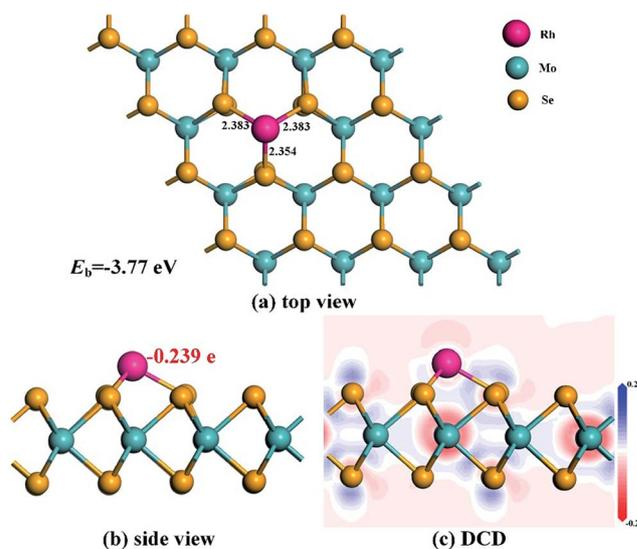
Fig. 1 Geometric structures (a) and (b) and DCD (c) of the Rh-MoSe<sub>2</sub> monolayer. The black values are the atom-to-atom distance while the red value is the electron amount carried by Rh dopant.
