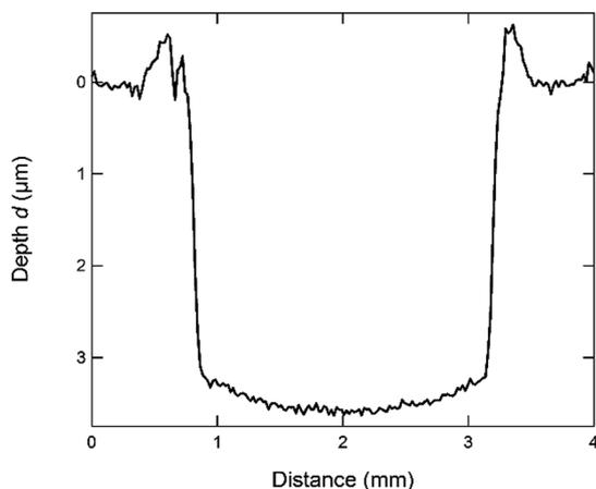
Fig. 1 Profilometer scan of a sputtered crater in a Mo/CIGSe layer stack. The image shows an average of 21 line scans taken within a distance of  $\sim 0.4$  mm in the middle of the file; moderate voltage and pressure were chosen in the present study.
