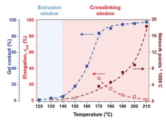
Fig. 5 Effect of temperature on hot set elongation ( $\square$ ), number of network points per 1000 C atoms ( $\blacksquare$  from hot set,  $\bigcirc$  from rheology), and gel content ( $\blacksquare$ ) for a 1.7:1 stoichiometric p(E-stat-GMA):p(E-stat-AA) blend cross-linked for 5 minutes; note that industrial standards for electrical insulation demand a hot set elongation of  $\varepsilon_{\text{hot}} = \lambda_{\text{hot}} - 100\% < 75\%$  for  $\sigma = 0.2 \text{ MPa.}^{42}$
