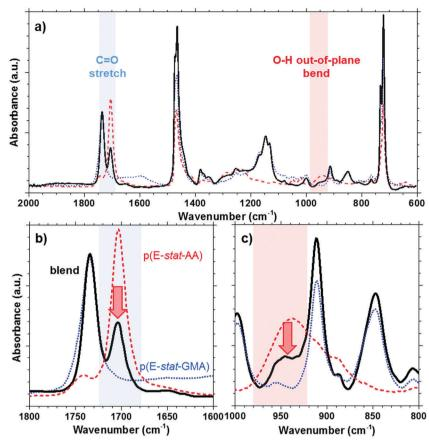
Fig. 3 (a) ATR-FTIR spectrum of the p(E-stat-AA):p(E-stat-GMA) polymer blend at stochiometric ratio; (b) reduction of the C=O stretching peak at 1705 cm<sup>-1</sup> upon blending; (c) reduction of the O-H out-of-plane bend peak at 940 cm<sup>-1</sup> upon blending; all spectra are normalized and p(E-stat-AA) and p(E-stat-GMA) intensities are scaled to their respective concentration in the blend; blend (solid); p(E-stat-AA) (dashed); p(E-stat-GMA) (dotted).
