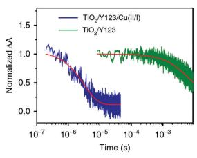
Fig. 9 Transient absorption spectra of Y123-sensitized photoanodes inert (green) and in contact with the solid Cu<sup>II/I</sup>(tmby)<sub>2</sub> hole transport material. Reproduced from ref. 87 with permission from the Nature publishing aroup
