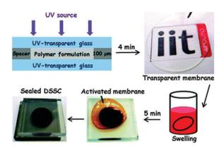
Fig. 21 Preparation of quasi-solid polymer electrolytes by swelling techniques. Reproduced from ref. 227 with permission from the Royal Society
