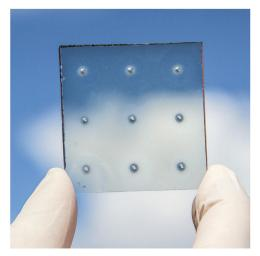
Fig. 27 Electropolymerized poly(3,4-ehtylenedioxythiophene) on an FTO substrate.
