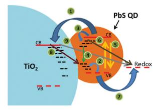
Fig. 19 Schematic illustration of photoinduced charge-transfer processes following absorption of quanta of light by PbS QDs on TiO2. Reprinted from ref. 190 with permission from the American Chemical Society.
