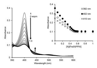
Fig. 5 UV-Vis titration of Fe(III)PPIX (2.4  $\mu$ M) with 1 in DMSO/33 mM HEPES buffer (pH 7.4) = 2 : 3 (v/v) at 25 °C. Inset: changes in the absorbance of Fe(III)PPIX upon the addition of 1.
