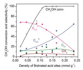
Fig. 11 Effect of density of Brønsted acid sites for the conversion of methanol over SSZ-13 zeolites. Reaction conditions: catalyst, 0.4 g;  $F(H_2) = 30 \text{ mL min}^{-1}$ ;  $F(\text{liquid CH}_3\text{OH}) = 0.01 \text{ mL min}^{-1}$ ; P = 2 MPa; T =673 K; time on stream, 3 h.
