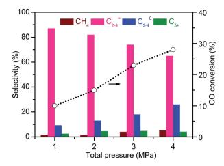
Fig. 9 Effect of total pressure of syngas on catalytic behaviours of Zn-ZrO<sub>2</sub>/SSZ-13-45H catalyst. Reaction conditions: catalyst, 0.60 g; H<sub>2</sub>/ CO = 2/1; T = 673 K; F = 30 mL min<sup>-1</sup>; time on stream, 10 h.
