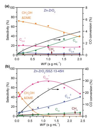
Fig. 8 Effect of contact time on catalytic behaviours of Zn-ZrO<sub>2</sub> and  $Zn-ZrO_2/SSZ-13-45H$  catalysts. Reaction conditions:  $W(Zn-ZrO_2) =$ 0.030-1.0 g;  $W(Zn-ZrO_2/SSZ-13-45H) = 0.030-1.2 \text{ g}$ ;  $H_2/CO = 2/1$ ; P = 3 MPa; T = 673 K;  $F = 30 \text{ mL min}^{-1}$ ; time on stream, 10 h.
