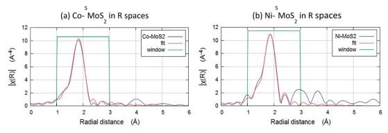
Fig. 6 Fourier transforms of the k3-weighted Co and Ni K-edge of extended X-ray absorption fine structure spectroscopy (EXAFS) spectra of (a) Co-SMoS<sub>2</sub> and (b) Ni-SMoS<sub>2</sub>
