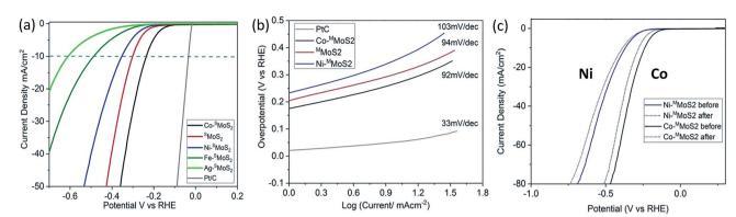
Fig. 2 HER activity analysis by linear sweep voltammography, LSV. (a) LSV of the  $M^{S}MoS_{2}$  nanosheets and the reference 20% Pt/C in 0.5 M  $H_{2}SO_{4}$  at a scan rate of 2 mVs<sup>-1</sup>. (b) Tafel plot of  $Co^{-S}MoS_{2}$ ,  $S^{S}MoS_{2}$ ,  $S^{S}MoS_{2}$ ,  $S^{S}MoS_{2}$  and  $S^{S$
