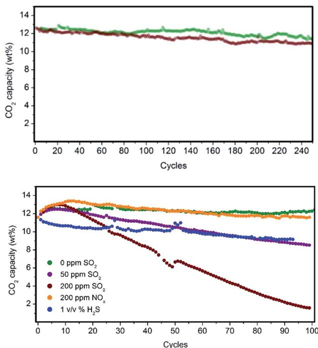
Fig. 6 (Top panel) Long-term CO<sub>2</sub> adsorption performance stability of PEI/(Zn)ZIF-8/SiO<sub>2</sub> (green) and PEI/(Zn)ZIF-7/SiO<sub>2</sub> (dark red) under simulated flue gas conditions. (Bottom panel) Long-term CO<sub>2</sub> adsorption performance stability of PEI/(Zn)ZIF-8/SiO<sub>2</sub> under the presence of SO<sub>2</sub>, NO<sub>x</sub> and H<sub>2</sub>S contaminants.
