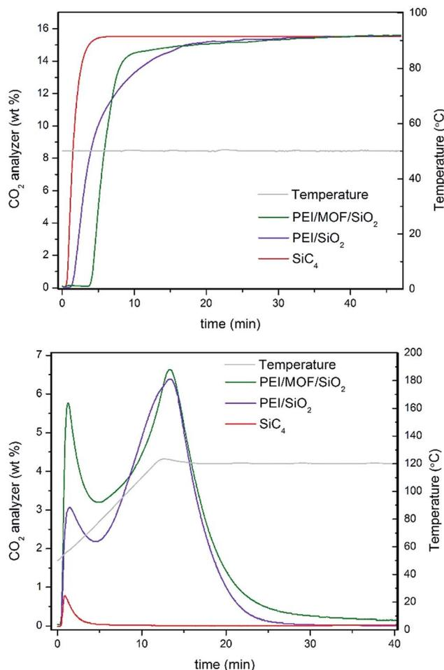
Fig. 5 (Top panel) Adsorption and (Bottom panel) regeneration profiles of 35 wt% of PEI/4.6 wt% of (Zn)ZIF-8/SiO<sub>2</sub> (entry 12, Table 1) and 35 wt% of PEI/SiO<sub>2</sub> (entry 1, Table 1).
