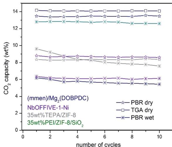
Fig. 3 CO<sub>2</sub> capture of polyamines impregnated on bulk MOFs compared with MOF/SiO<sub>2</sub> under simulated flue gas conditions in a PBR.
