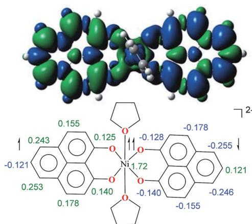
**Fig. 3** The spin density plot for **2**, where the colour coding refers to green = excess  $\alpha$  spin and blue = excess  $\beta$  spin. The contour values were set to  $\pm 0.0004$  (e bohr<sup>-3</sup>)<sup>1/2</sup> (above). The major numerical values of excess spin densities are shown (below).
