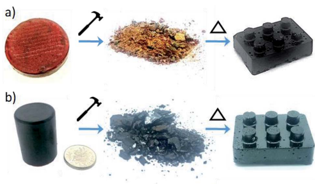
Fig. 6 Sulfur polymer samples on, after breaking into powder, centre, and then after being reformed into a monolith again, right: (a) sulfur–perillyl alcohol copolymer, and (b) sulfur–squalene copolymer. Both samples were made with 50 wt% sulfur.
