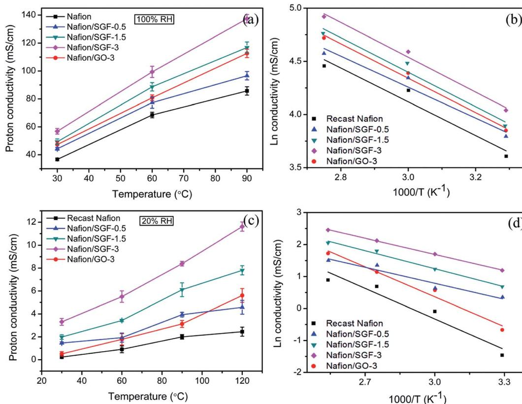
**Fig. 7** Temperature variant proton conductivities of pristine recast Nafion and composite membranes (a) under 100% RH and (c) under 20% RH; corresponding Arrhenius plots of proton conductivities (b) under 100% RH and (d) under 20% RH.
