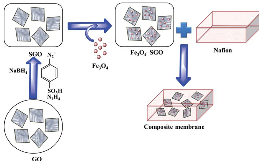
Scheme 1 Preparation process of Nafion/Fe<sub>3</sub>O<sub>4</sub>-SGO composite membrane.
