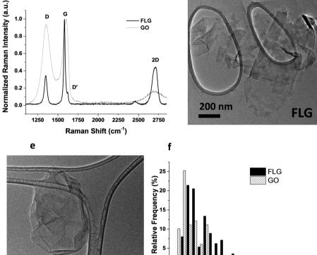
Fig. 1 Physicochemical characterization of the GO and FLG used in this study. (a) Thermogravimetric analysis, (b) elemental analysis, (c) Raman spectroscopy, (d-e) TEM images, (f) lateral size distribution from TEM observations.
