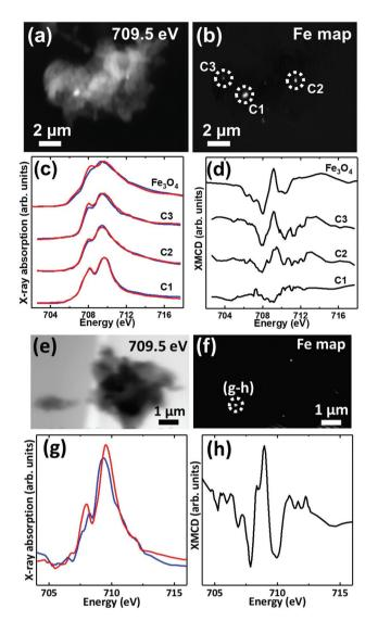
Fig. 7 (a, e) X-ray microscopy images (b, f) iron  $L_3$  edge speciation maps (c, g) X-ray absorption spectra and (d, h) XMCD spectra from an APC of case X. Panels (c) and (g) show X-ray absorption spectra obtained using LCP (blue spectra) and RCP (red spectra). Panels (d) and (h) show the corresponding XMCD spectra created by subtracting the RCP spectra from the LCP spectra. All spectra were obtained in a magnetic field of  $\sim$ 150 mT applied parallel to the incident X-ray beam.
