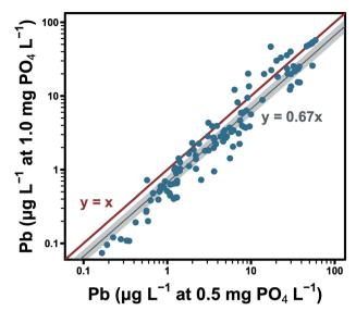
Fig. 2 System A and B lead concentrations at 1.0 mg PO<sub>4</sub> L<sup>-1</sup> were an estimated 67% of concentrations at 0.5 mg  $PO_4$   $L^{-1}$  (paired measurements at 17 residences comparing Apr. 2016 with an average of Dec., Mar., and Apr. 2017). The gray shaded region represents the 95% CI around the group difference estimate of 0.67.
