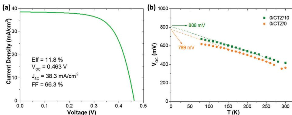
Fig. 7 (a) *J*–*V* curve corresponding to the best solar cell obtained in this work. (b)  $V_{OC}$  vs.  $T$  plot of a reference sample without Ge and a sample with 10 nm of Ge deposited on top of the CTZ precursors.
