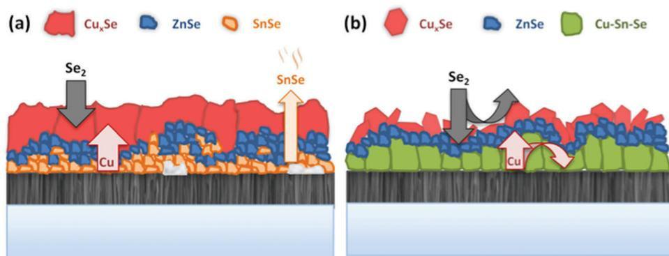
**Scheme 2** Schematic sketches of the different intermediate steps and reaction mechanisms involved in the formation of CZTSe during the selenization of metallic Cu–Zn–Sn precursors: (a) reference sample without Ge, and (b) Ge-containing sample.
