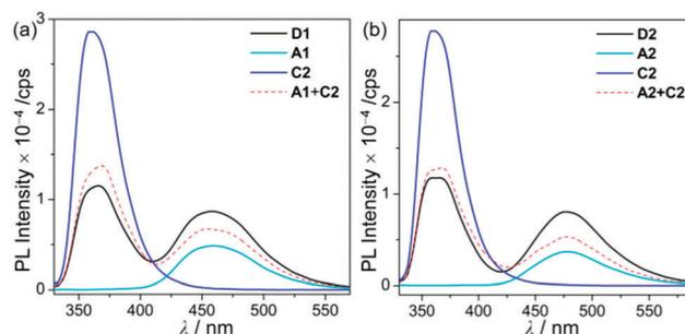
Fig. 3 PL spectra in THF ( $5.0 \times 10^{-5}$  M) for (a) **D1**, **A1**, and **C2** ( $\lambda_{\text{ex}} = 310$  nm) and (b) **D2**, **A2**, and **C2** ( $\lambda_{\text{ex}} = 316$  nm) at room temperature.
