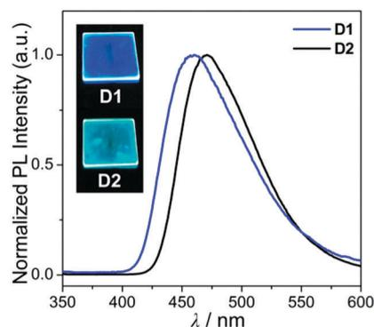
Fig. 4 PL spectra of the film (5 wt% doped on PMMA) for **D1** and **D2**. The insets are photographs of the film under a handheld UV lamp ( $\lambda_{\text{ex}} = 365 \text{ nm}$ ).
