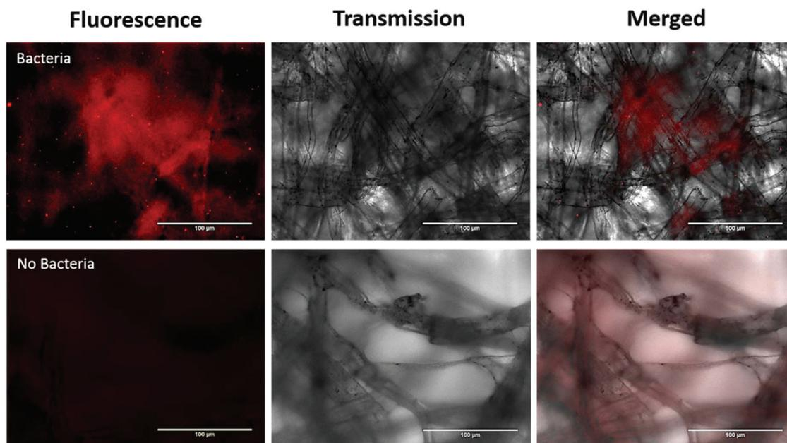
**Fig. 4** Fluorescence images showing bacteria on AuNP-paper substrates. Bacteria were treated with Syto60 ( $5 \mu\text{M}$ ), the top row consists of AuNP-paper containing bacteria, merged, transmission, and fluorescence images. The bottom row corresponds to AuNP-paper without bacteria.
