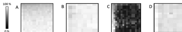
Fig. 1 MALDI images of square areas (150 \times 150 \text{mm}^2 ) showing homogeneous desorption/ionization behaviour of dithranol over each area with the exception of the sample on polyimide tape at a step size of 100 \times 100 \mu\text{m} (C) showing reduced intensity after the first line. Dithranol was applied by sublimation on double-sided tape (A and B) and polyimide tape (C and D). Step size 100 \times 100 \mu\text{m} (A and C) and 150 \times 150 \mu\text{m} (B and D). Images are TIC normalized. Intensity scale bar shows relative intensities.
