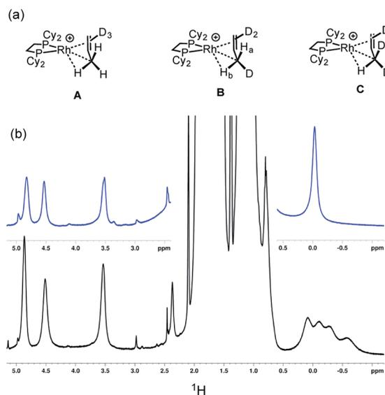
Scheme 9 (a) Isotopomers  $[\mathbf{1}\text{-}(\text{d}_3\text{-propene})][\text{BAR}^{\text{F}}_4]$  highlighting the methyl substitution patterns. (b)  $^1\text{H}$  NMR spectra (193 K,  $\text{CD}_2\text{Cl}_2$ ) of a sample prepared by the solid/gas route after 16 hours. Top,  $[\mathbf{1}\text{-}(\text{propene})][\text{BAR}^{\text{F}}_4]$ ; bottom,  $[\mathbf{1}\text{-}(\text{d}_3\text{-propene})][\text{BAR}^{\text{F}}_4]$ .
