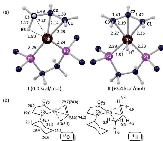
Fig. 4 Computational characterization of [1-(propene)][BAR<sup>F</sup><sub>4</sub>] in the solid-state: (a) structures of the molecular cation in its [1-(propene)]<sup>+</sup> and [1-(allyl-hydride)]<sup>+</sup> forms (I and II respectively, selected distances in Å; truncated Cy groups); (b) computed <sup>13</sup>C and <sup>1</sup>H data for the [1-(propene)]<sup>+</sup> cation, with selected <sup>13</sup>C experimental data (SSNMR, 158 K) in parenthesis.
