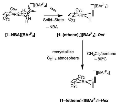
Scheme 4 Synthesis of [1-(ethene)<sub>2</sub>][BAR<sup>F</sup><sub>4</sub>] as octahedral ("Oct", *C*<sub>2</sub>/*c*) and hexagonal ("Hex", *P*<sub>6<sub>3</sub>22) polymorphs.</sub>
