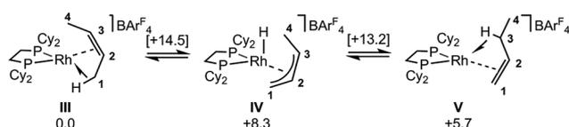
Scheme 12 Computed mechanisms for interconversion of [1-(*cis*-2-butene)]<sup>+</sup>, III, and [1-(1-butene)]<sup>+</sup>, V, cations in the solid-state. Free energies are indicated in kcal mol<sup>-1</sup> with those for transition states provided in square brackets.
