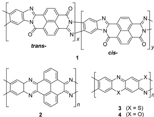
Fig. 3 Chemical structures of *trans* and *cis* poly(benzimidazole benzophenanthroline) (BBL) **1**, polyquinoxaline (PQL) **2**, poly(phentiazine) (PTL) **3**, and poly(phenoxazine) (POL) **4**.
