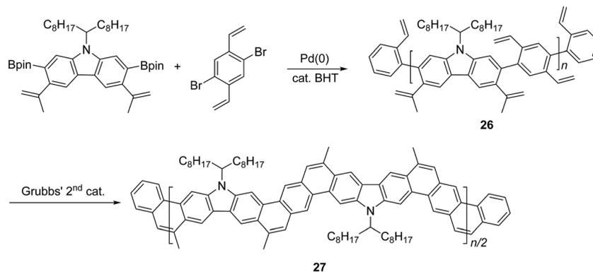
Scheme 11 Synthesis of carbazole-based ladder polymer 27 by thermodynamically controlled ring-closing olefin metathesis.
