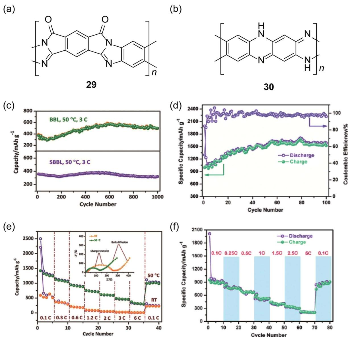
Fig. 10 Chemical structures of (a) SBBL **29** and (b) PQL **30**. Electrochemical performance of ladder polymer nanoparticles. Cycling performance of (c) BBL **1**, SBBL **29** and (d) PQL **30** nanoparticles showing their superb stability. Rate capability of (e) BBL **1**, SBBL **29** and (f) PQL **30** nanoparticles. Reproduced from ref. 107 and 108 with permission from John Wiley and Sons.
