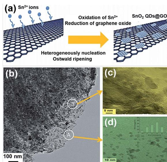
Fig. 2 (a) Schematic illustration for the fabrication of SnO<sub>2</sub> QDs@GO. (b) TEM image of SnO<sub>2</sub> QDs@GO. (c), (d) High-resolution transmission electron microscope (HRTEM) of section B and A in image (b), respectively. The inset in image (d) is a size distribution image. Reprinted with permission from ref. 47. Copyright 2015 Wiley-VCH.
