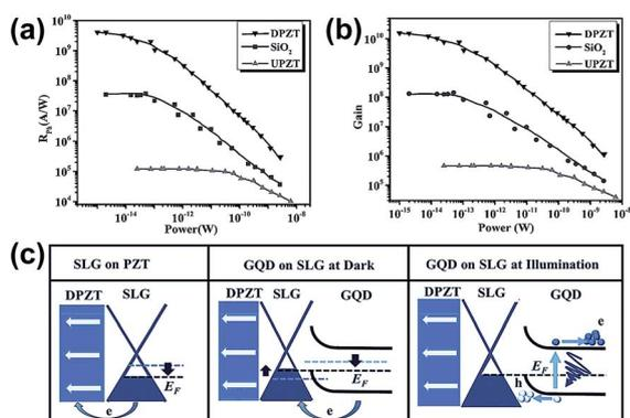
Fig. 12 Photoresponsivity ( $R_{ph}$ ) (a) and photocurrent gain (b) as a function of applied power for different substrates. (c) Schematic energy band diagrams for different devices and conditions. Reprinted with permission from ref. 92. Copyright 2015 WILEY-VCH Verlag GmbH & Co. KGaA.
