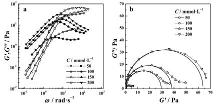
Fig. 4 (a) Dynamic rheological spectra and (b) the Cole-Cole plots of the di-Ph-C16/N-2-N system (filled and open symbols in (a) represent the elastic modulus (G') and viscous modulus (G''), respectively)
