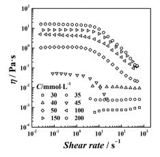
Fig. 2 Steady shear viscosity curves of di-Ph-C16/N-2-N at different Ph-C16 ion concentrations.
