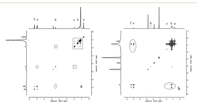
Fig. 7 The 2D NOESY spectra of the (a) sodium Ph-C16 and (b) di-Ph-C16/N-2-N systems (concentration of Ph-C16 ion: 5 mmol  $L^{-1}$ ).
