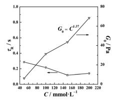
Fig. 5 The relaxation time,  $\tau_{\rm R}$ , and plateau modulus,  $G_0$ , of the di-Ph-C16/N-2-N systems as a function of the Ph-C16 ion concentration.
