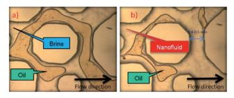
Fig. 4 Flooding experiment carried out with microfluidic chip (a) brine flooding (b) silica particle nanoflooding. Hendraningrat *et al.* concluded that nanofluid can potentially increase recovery rate. (Reprinted with permission from (ref. 48). Copyright (2013) Elsevier.)
