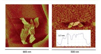
Fig. 2 PFM images (topographical map) of TPPS<sub>3</sub>NH<sub>2</sub> aggregates deposited on highly ordered pyrolytic graphite (HOPG) from an  $8.8 \times 10^{-5}$  M aqueous solution of the porphyrin at pH = 4.0 (HCl). The inset shows the height analysis of the section of the spiral structure folded so as to form bilayered regions.
