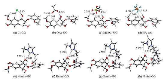
Fig. 1 Optimized anion-GG conformers (a-d), and cation-GG conformers (e-h) at the level of  $6-31++g^*$ . H-Bonds are indicated by dashed lines.
