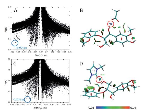
Fig. 2 RDG scatter plots (isovalue = 0.5 a.u.) and surface plots (s = 0.7 a.u.) of (A and B) OAc-GG interaction and (C and D) Mmim-GG interaction. The isosurfaces are colored on a blue-green-red scale according to values of  $sign(\lambda_2)\rho$ , ranging from -0.03 to 0.02 a.u. Blue indicates strong attractive interactions and green indicates the  $\pi$ -stacking interaction.
