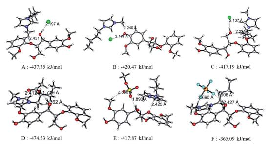
Fig. 4 Optimal structures of interaction between GG and Bmim based ILs at B3LYP/6-31++g\*\* level and H bonds are indicated by dashed line. Structures (A), (B), and (C) are BmimCl-GG interaction at  $\alpha$ , p, and  $\gamma$  position respectively. Structures (D), (E) and (F) are BmimOAc-GG, BmimMeSO<sub>4</sub>-GG, and BmimPF6-GG interaction at  $\alpha$  position.
