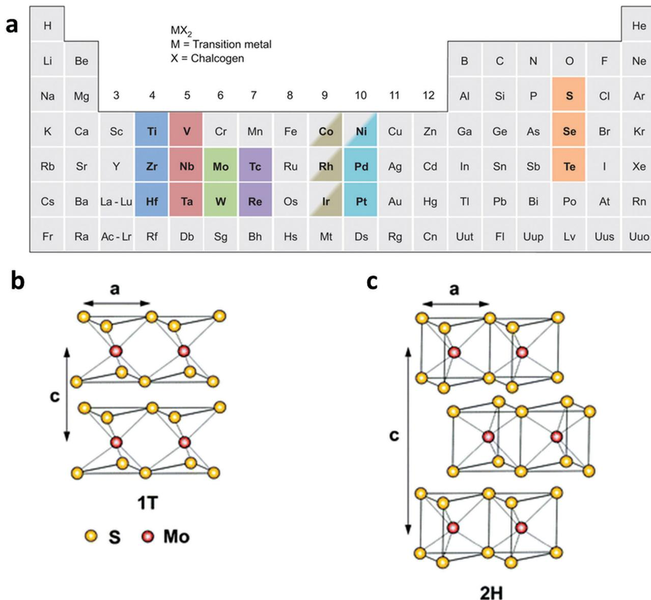
Fig. 1 (a) Various kinds of TMD nanomaterials, reproduced with permission from ref. 20. Copyright 2013 Nature Publishing Group. Schematic illustration of (b) the 1T-type and (c) the 2H-type structure of MoS<sub>2</sub>. Reproduced with permission from ref. 8. Copyright 2013 Royal Society of Chemistry.
